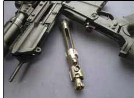
The integral striker plate is machined into the bolt carrier versus being screwed to the bolt carrier like a traditional AR. Grooves in the bolt carrier allow sand and other foreign matter to pass through without jamming or producing sluggish operation, which translates to greater reliability in adverse conditions. The charging rod can be seen here in the rearward position. The charging handle is located on the left side of the rifle.
