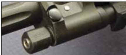
The heart of the system begins with the finely variable gas block. The knob at the forward end of the block can be turned for different bullet weights or for sluggish operation, but primarily for tuning barrel harmonics. How the gas drives the bolt carrier and how the gas is expelled required many months of design, redesign, and testing on the range to overcome what has been a challenge in previous DI systems. Note here also that additional accessory rails can be added to the forearm.
