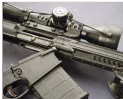
Fit up of the forearm and barrel is unique. It is a major factor in the rifle's accuracy. The receiver also has a spent brass deflector.
