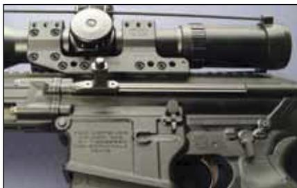
The charging handle is located on the left side of the upper receiver. From it protrudes a button, which is used as a forward assist. Place the big knuckle of your index finger on the button and depress it, grasp the handle, and with your thumb, move the charging handle forward.
